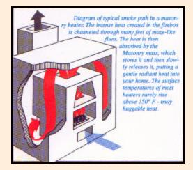
Think of a masonry heater as a large warm rock in the middle of your home. It's a high mass heat storage system. Short, hot fires generate tremendous amounts of heat which is then stored into the masonry, to be slowly and evenly released into your home.
